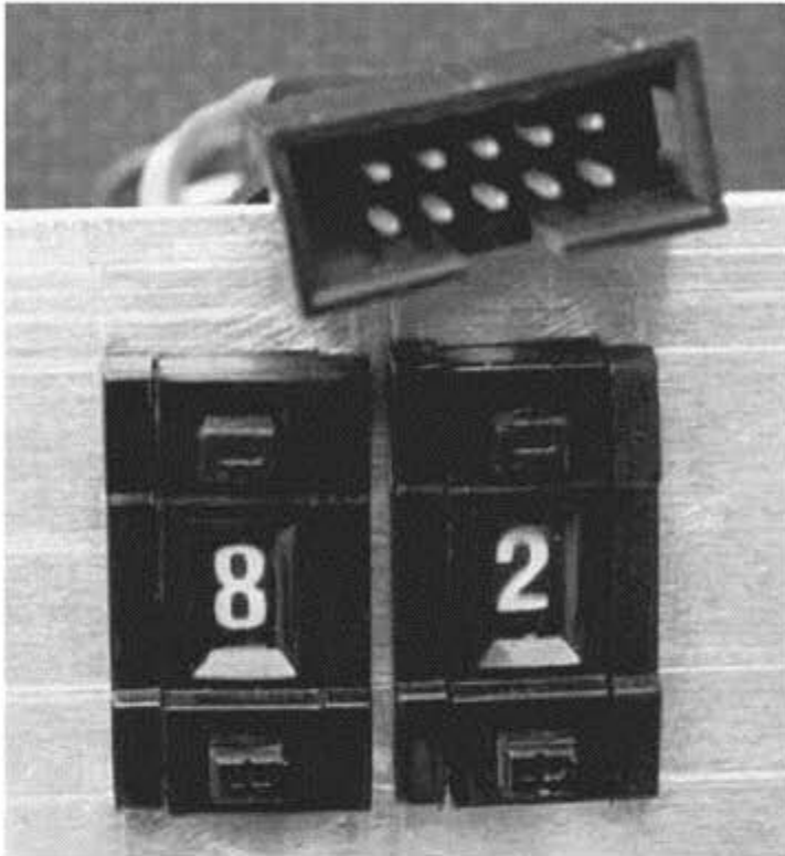
FIGURE 13.4 Photograph of a pair of thumb-wheel switches
