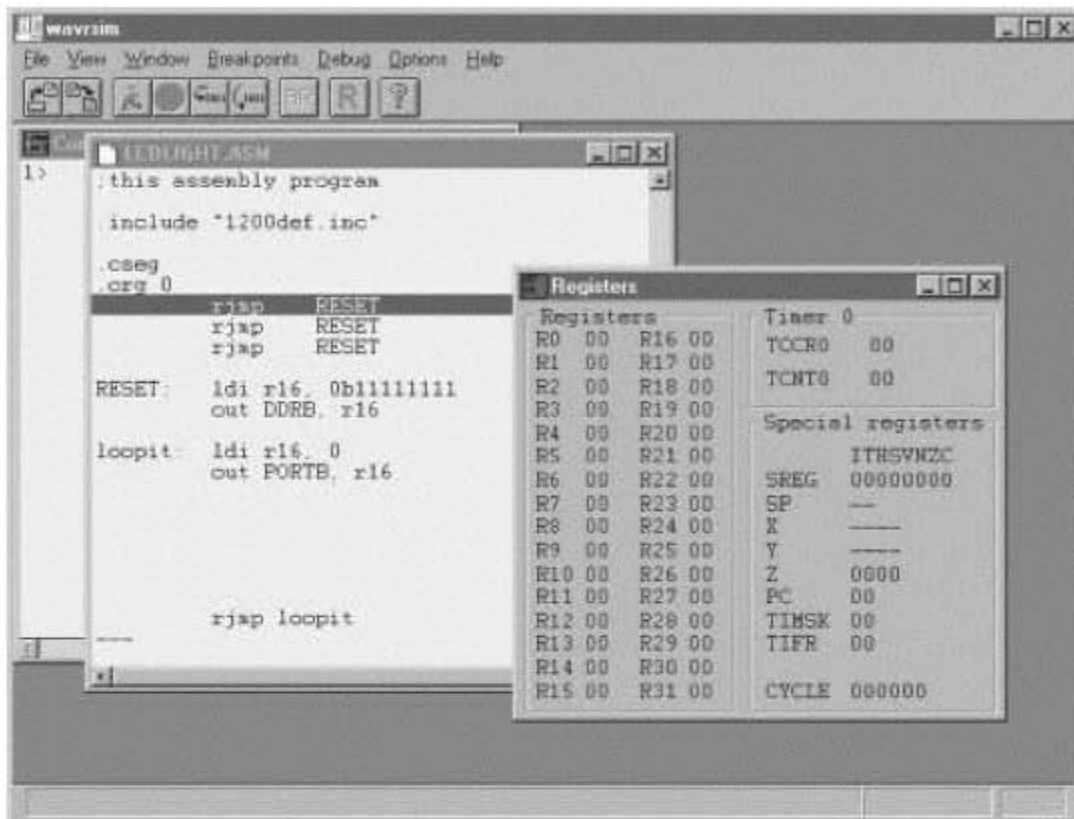
FIGURE 8.2 The AVR Simulator.
